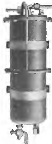
Sparton vacuum fuel feed tank which incorporates two chambers, the upper for suction and the lower for discharge. Only 5 sec. of cranking is required to fill the tank when empty
